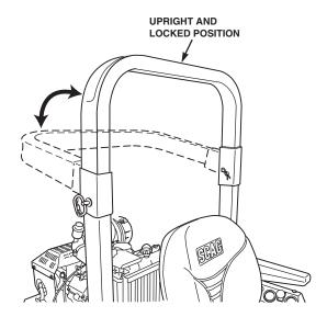
Figure 2-1. Foldable Roll-Over Protection System
